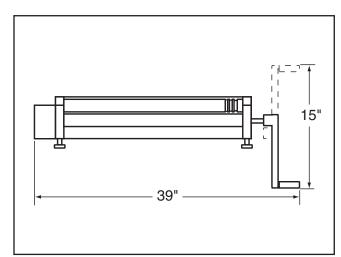
Figure 5. Minimum working clearances.
